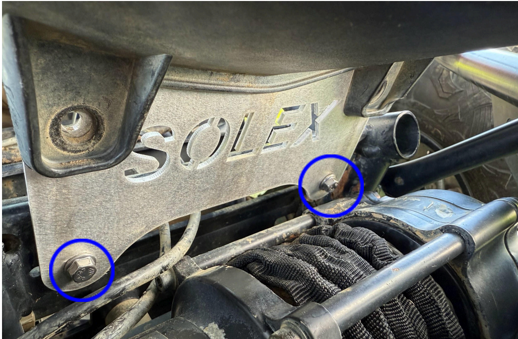
Shown above: Installed bottom frame bolts (M6x16mm)
