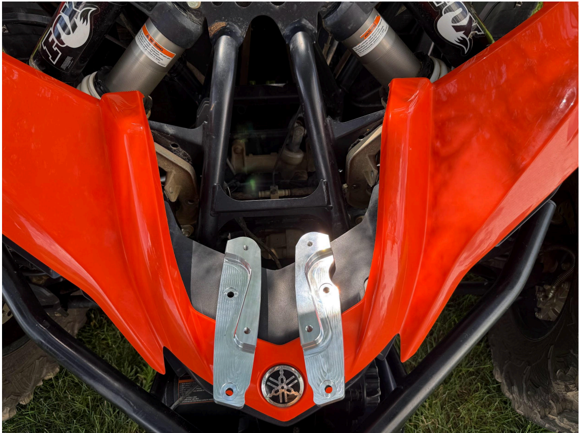
Shown Above: Right and Left machined headlight brackets (respectively)
