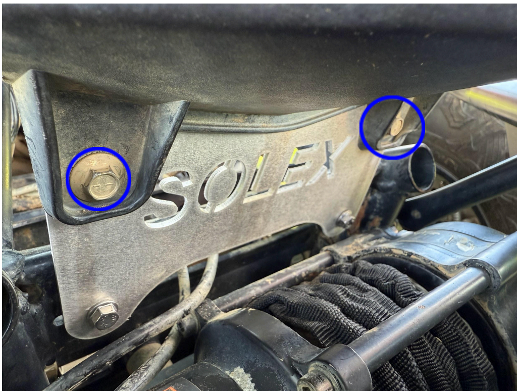
Shown above: Installed headlight housing bolts (supplied M6x20 bolts with flanged polymer washer and locking nuts on back)
