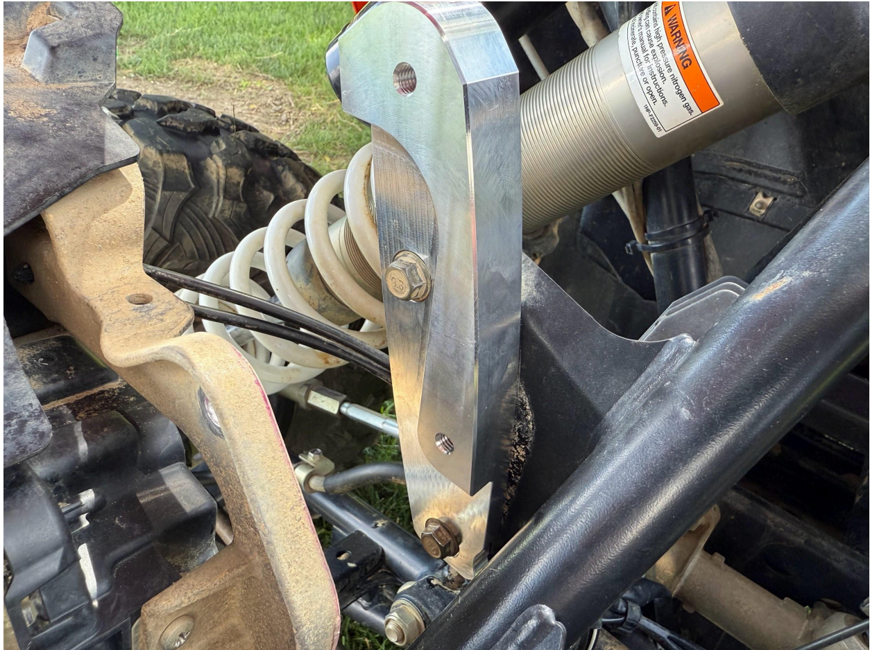
Shown above: Right headlight bracket installed
