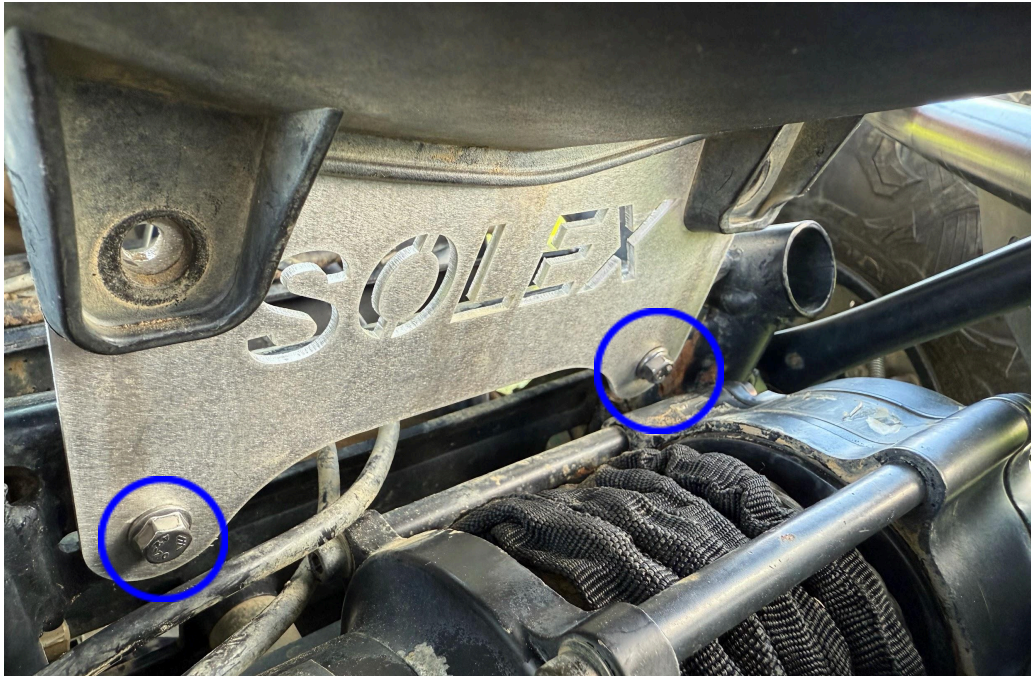
Shown above: Installed bottom frame bolts (M6x16mm)
